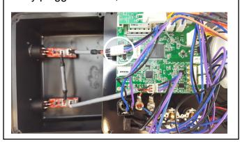
**Step 10)** Connect the 6" XLR cable into the J5 connector on the Audio Box board.
