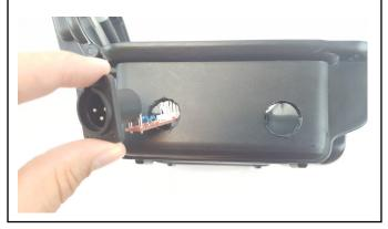
**Step 6)** Use drill to insert screws into top left and bottom right of each XLR connector.
