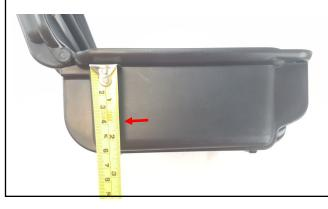
Step 4) Drill hole into the left side of case using 13/16" spade bit. Repeat for right side.
