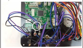
**Step 9)** Connect the cable that was previously plugged into J5, into male XLR cable.
