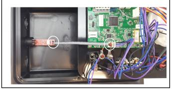
**Step 9)** Connect the cable that was plugged into J5 on the Audio Box, into the CN3 connector on the XLR board.
