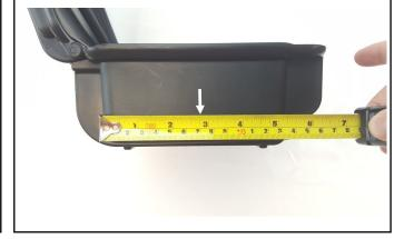
**Step 3)** Measure and mark 1 1/2" down from the bottom lip of the armored case.
