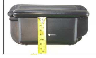
**Step 4)** Using the marks from steps 2 & 3, drill into the middle of the case using the 13/16" spade bit.
