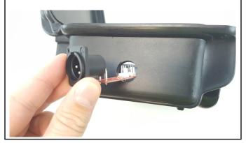
**Step 6)** Use the drill and phillip bit to insert the included screws into the top left and bottom right of the XLR connector.
