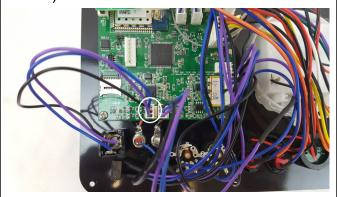
**Step 8)** Connect the XLR cable into the J5 connector on the Audio Box and the CN2 connector on the XLR board.
